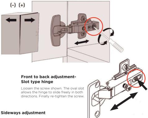
Sideways adjustment of the door is done by turning the screw shown in either direction.
